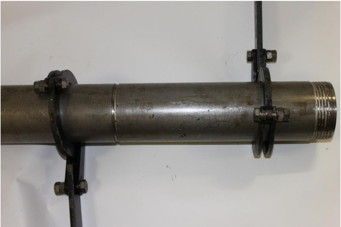
Figure 6. Wrenches to disassemble tubes and bit.
